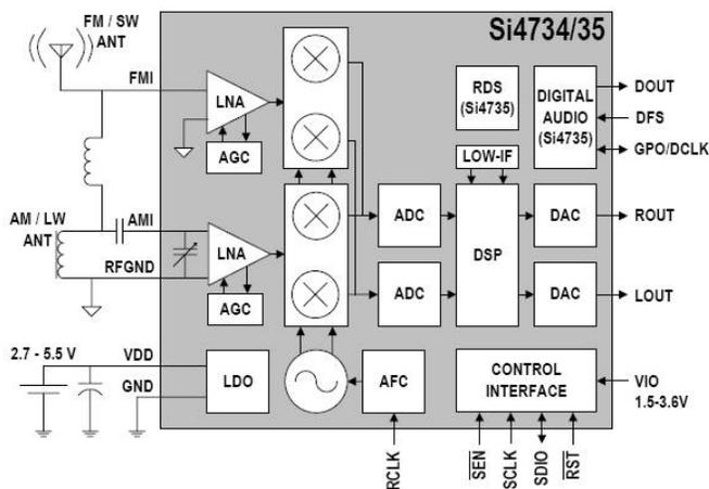
As can be seen in the functional block diagram at left, a manufacturer only needs to provide a power supply, an antenna input, a display and a final audio section for sound, while the DSP chip takes care of all other receiver-related functions.
