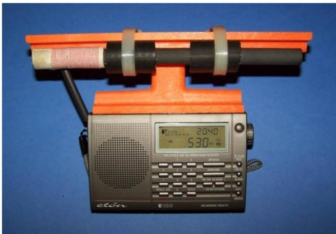
A comparison of the G8, Eton e100 (left) and C Crane SWP with identical eight-inch external ferrite antennas shows that the G8 had the greatest sensitivity of the three by a small margin. As noted above, the Eton and C Crane models, when fitted with narrow Murata filters, are still superior when receiving split-frequency trans-oceanic signals. [Further information](#) is available regarding the modification of the G8 and other radios in this way.
