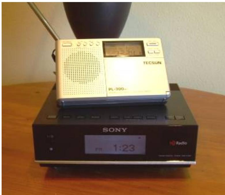
As for selectivity, detuning 0.1 MHz on both sets showed that the Sony's adjacent channel selectivity figure (80dB) is clearly better than that of the G8 (50 dB). However, in all my tests, the extra 30 dB of selectivity was never an issue, in that the G8 was always able to separate stations spaced 0.2 MHz apart. For those in Europe and other locations where you actually have stations 0.1 MHz apart, the Sony may really shine, but here near Seattle, there was not a noticeable difference.
