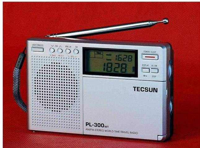
The radio measures 135 x 86 x 26 mm. (about 5.3 x 3.4 x 1 inches), which just barely fits into my shirt pocket, and so likely represents the largest that a radio could be and still be an Ultralight. It weighs 204 grams (about 7 ounces), which is typical for an ULR. It comes with a nice zippered travel case.
