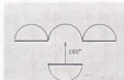
Fig. 3—Phase of the current in high band dipole changes 180 degrees as it travels to the point in space where it is ahead of the two outer dipole sections.
