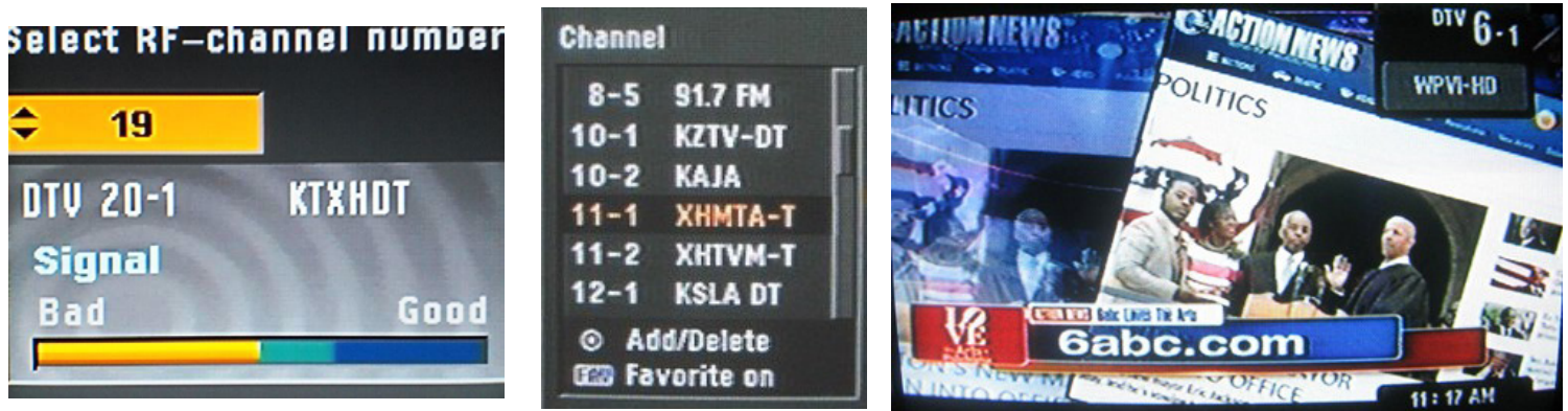
(Left) This is the manual tuning screen of a Zenith DTT-901. The “19” in the yellow box is the RF channel, while the “DTV 20-1” is the virtual channel. “KTXHDT” is the station ID. Note the signal strength bar across the bottom. (Center) This channel list is from a Zenith DTT-901. Those numbers are virtual channels. For example, XHMTA’s RF channel is actually 12. (Right) At a distance of 1,157 miles, digital WPVI-DT, channel 6 (virtual channel 6) in Philadelphia is a regular summertime catch for me. (Courtesy of the author)
