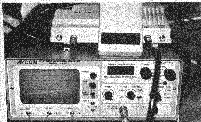
PROPER analysis of amplifier bandpass characteristics requires a frequency-identifiable “sweep.” Here, a Promax NG72 broadband noise bridge is fed to an Alcad CF711 amplifier and the detected response is displayed in a frequency-spectrum that covers 40 - 900 MHz. The (as adjusted) amplifier “tilt” is apparent in the display on the screen; covering 47 (left side) - 862 MHz (right side) over a 18 dB range.
