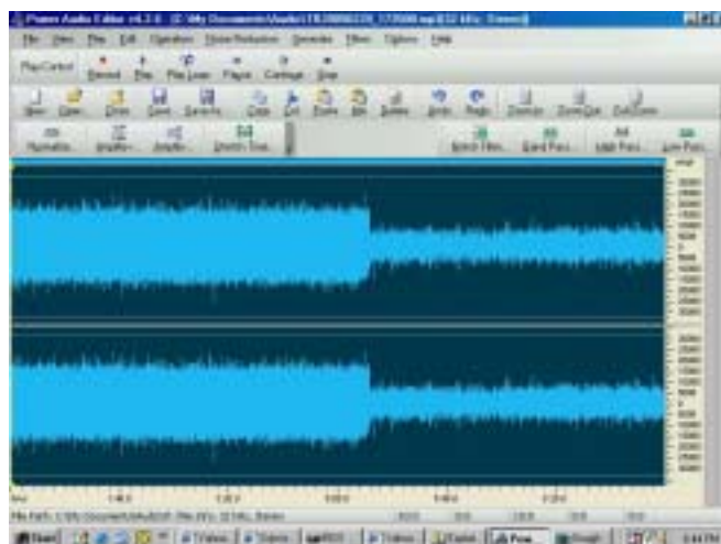
This is for you AM fans. It is a graphical representation of the IBOC first-adjacent sideband on 960 kHz. From local WPEN-950 as the IBOC signal is turned off at local sunset. This was recorded @ 1730 EST on 2/20/05.
