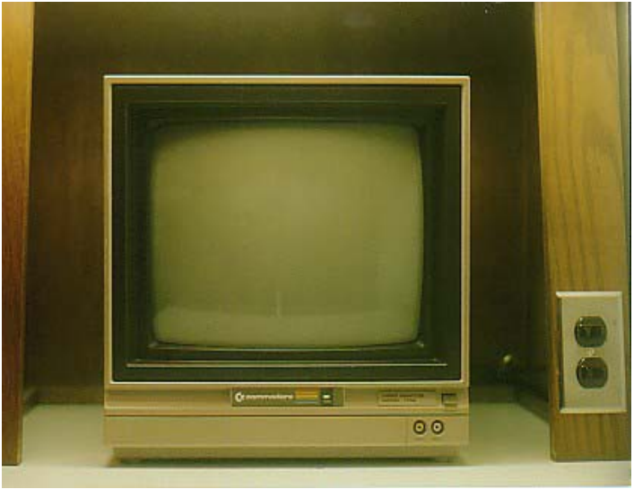
1984 Commodore color monitor (model 1702) used for taking photos ("richer color and sharper images, especially for weak ID's")
