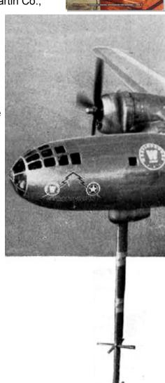
The experimental Stratovision station (a modified B-29). flying at 25,000 feet over the Pittsburgh area, rebroadcast telecast picked up from the east coast television network over an estimated area 525 miles in diameter. Programs from the ground stations are picked up on the antenna projecting above the tail. and rebroadcast from the long. mastlike antenna extending down from the nose of the plane.
