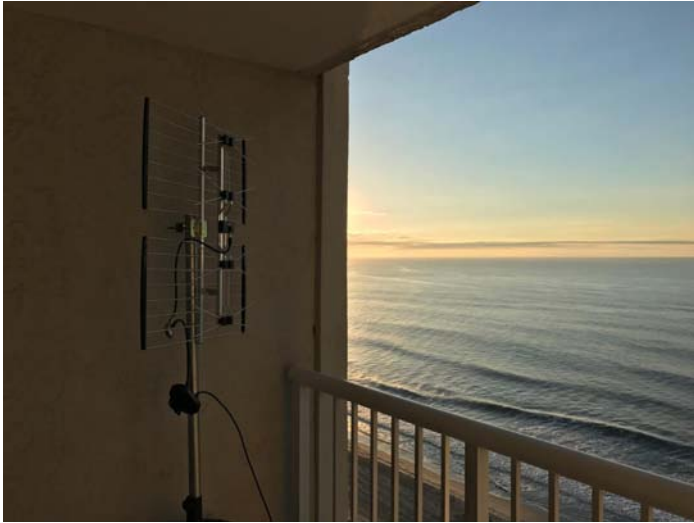
The setup: 4-bay on 11 th floor + direct water path ...
