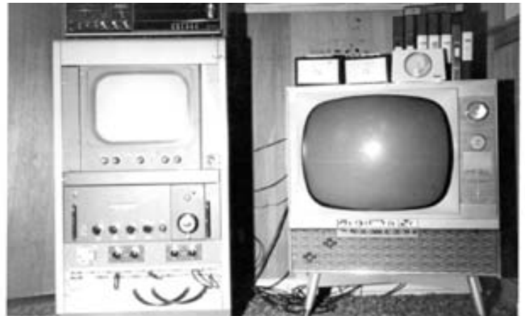
TV setup in Deerfield, Illinois. The rack on the left had wave traps and a patch panel along with a Conrac tuner (which had been recommended by Bob Cooper) and a black and white video monitor. Note I had 3 rotors hooked up for all the antennas. (see next page)
