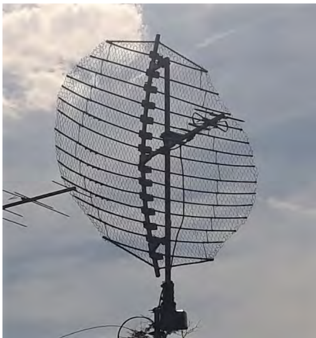
And here's the antenna that gets it all – the rebuilt Finco P-5 dish at a temporary height of 11 feet agl.
