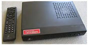
box (both labels, Zenith and Insignia) in the 2008-2009 transition. The receiver's sensitivity is good (noise figure of around 6 dB) and good multipath performance (probably using a frequency domain equalizer).
