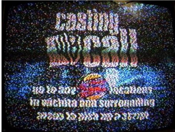
Tropo on UHF in the analog era: KWCV 33 Wichita, KS (now KSCW) 400 miles (660 km), as seen on July 19, 2003
