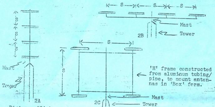
Distance 'S' is again the distance between antennas. Now we use a four way hybrid mixer because we have four antennas to combine. The mixer should be mounted in a central location, and all connecting cables from antennas to the mixer once again exactly the same length. The two closest antennas will have excess cable, and this should be coiled neatly and taped to the support mast close to the hybrid mixer; not at or near the antenna(s). Vertical stacking distances are now
