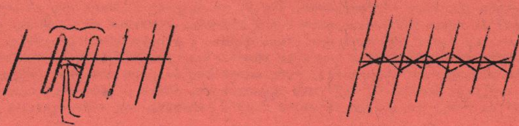
8a) Yagi; only driven elements are interconnected.
