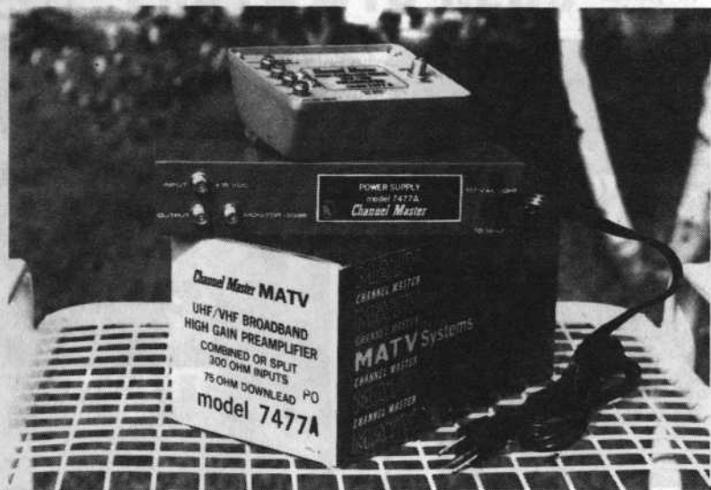
High performance Channel Master MATV preamplifier 7477A is mated with Winegard's top-of-the-line Chromstar UHF antenna, CS-9095. The 7477A's 300-ohm inputs and 75-ohm output eliminates the need for an antenna-mounted balun. Power supply and preamp housings are constructed of heavy-gauge metal.
