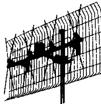
Figure 3: A grid aerial, shown mounted for vertical polarisation
